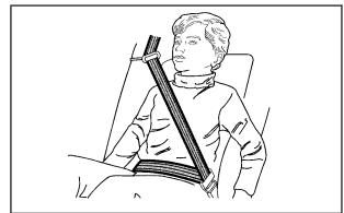
Buckle, position and release the safety belt as described in *Rear Seat Passengers on page 1-22*. Make sure that the shoulder belt crosses the shoulder.
